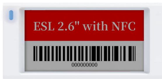
(ESL label 2.6" with a resolution of 296 x 152 dots and three colors black, white and red)
